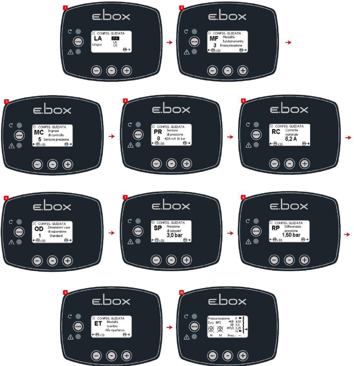
Figure 12: Configuration with a pressure sensor
