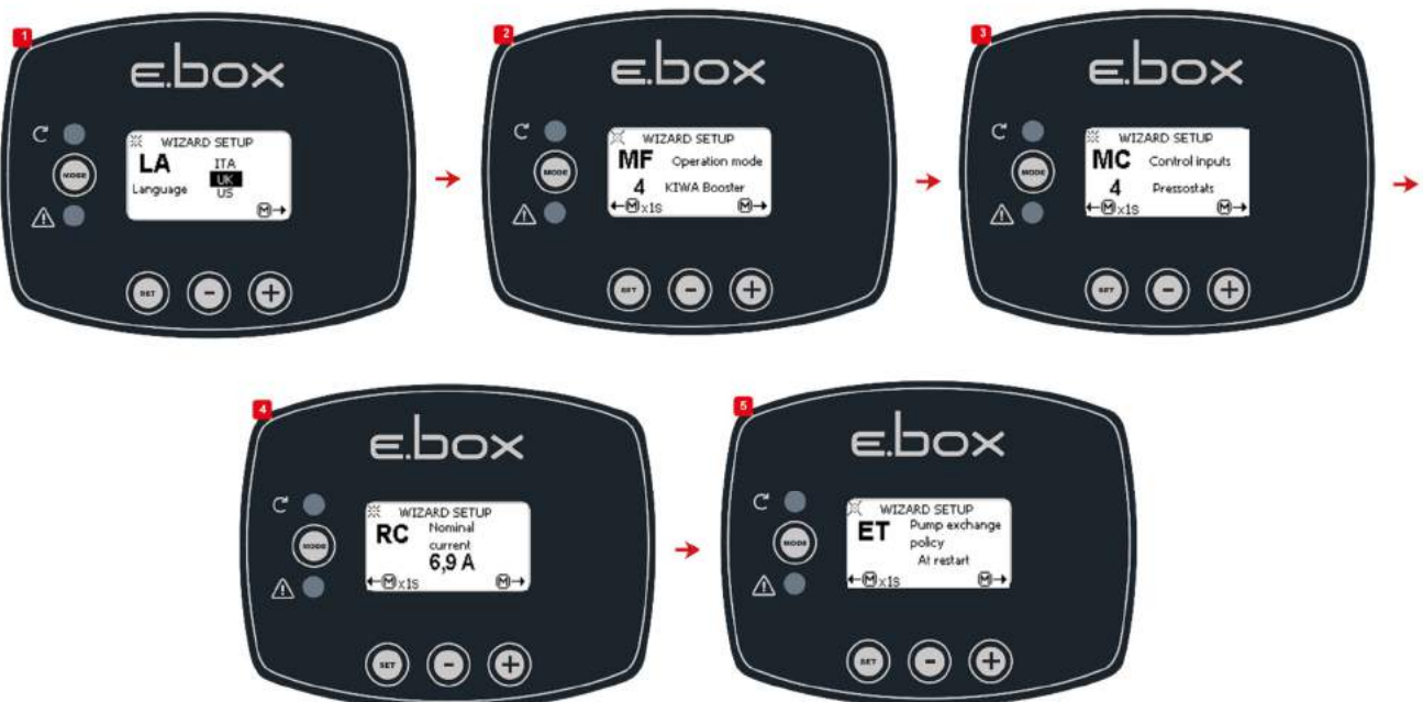
Figure 49: Kiwa configuration with pressure switches
