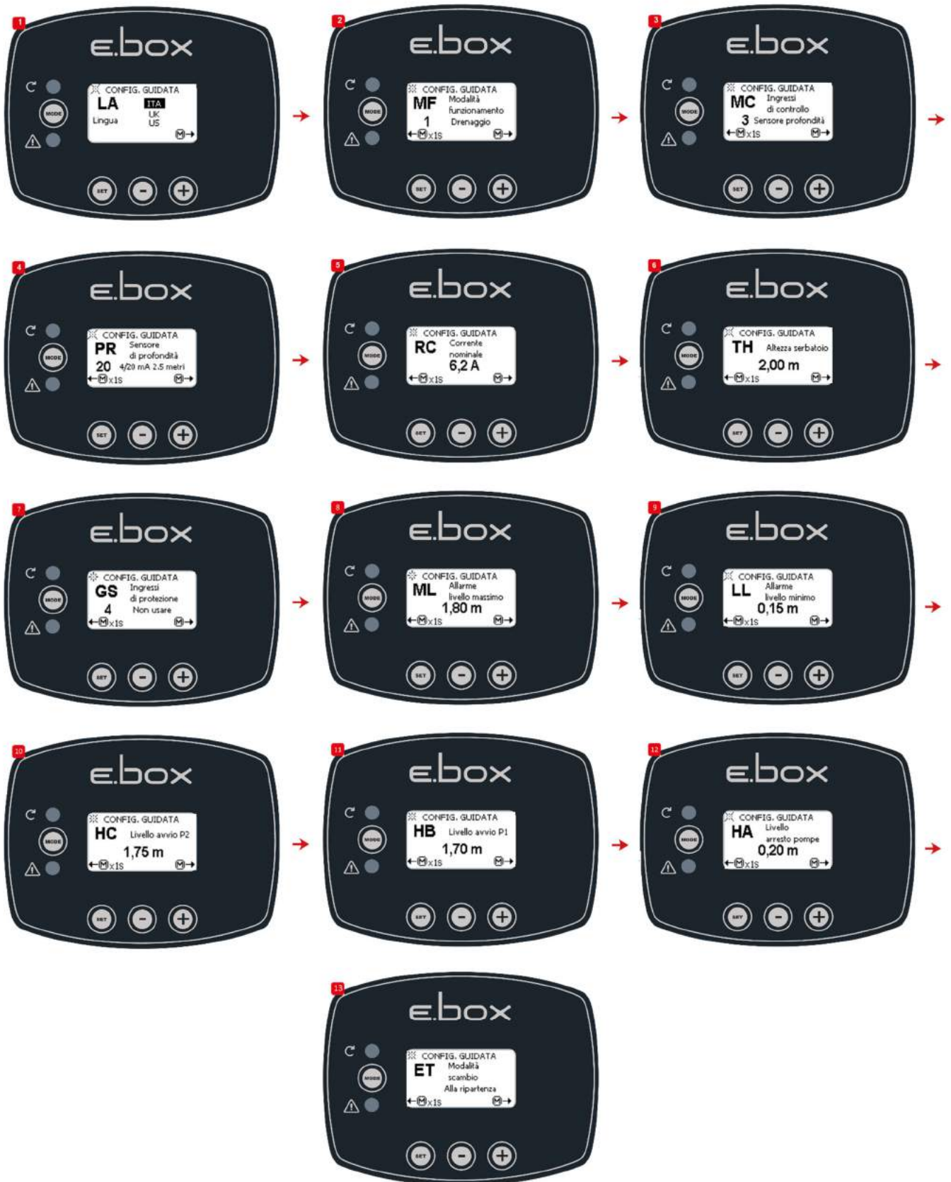
Figure 38: Configuration with only a depth sensor
