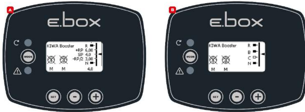
Figure 50: System status in KIWA mode
