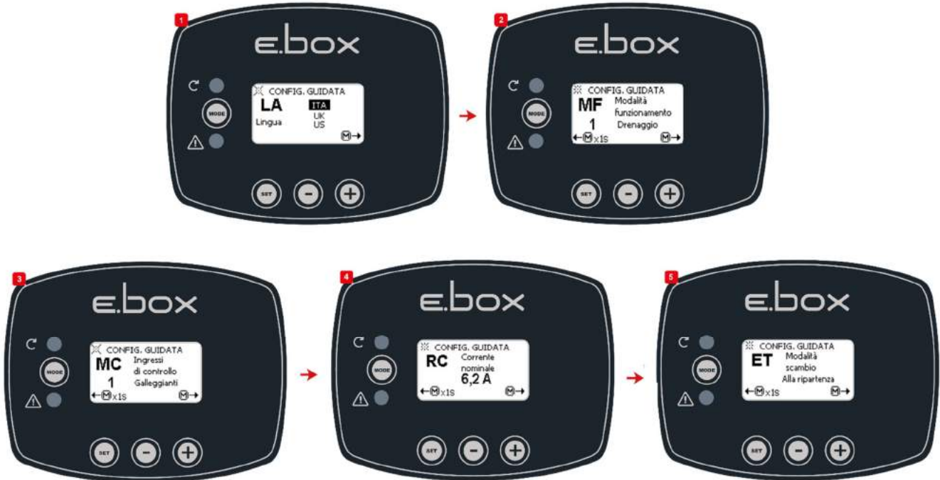
Figure 36: Configuration of Drainage floats or level probes
